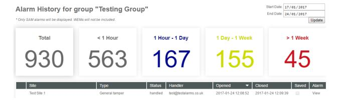
Excessive alarm activity from the same device can indicate that the system is not functioning correctly. In this case, a site visit is recommended.
