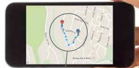
ALARM RECIPIENT'S PHONE(S) Once activated the worker's movements are shown in real time on the map displayed in a browser or enabled smartphone
